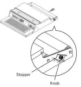
After adjustment, to keep the brake knob firmly fixed, turn the stopper clockwise and tighten it to secure the knob.
