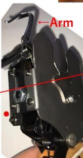
• The screw and nut marked with • are used for adjusting the arm height. Untighten the nut, then adjust the position of the screw.
